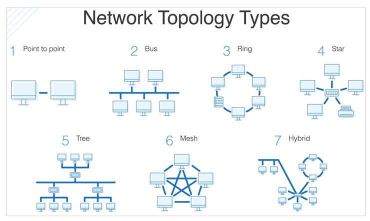
Network topology diagrams aid the computer network design process. Source: www.dnsstuff.com.
